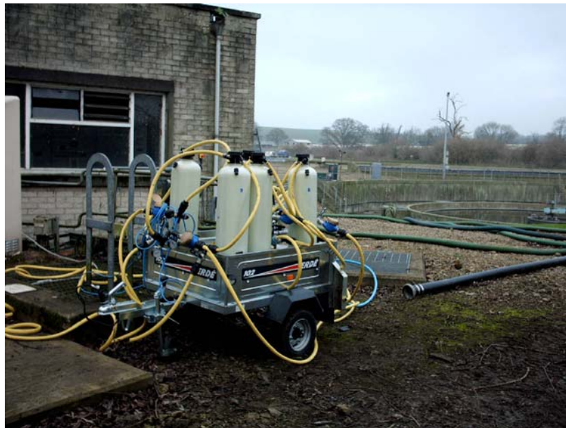
Figure 7. The pilot rig comprising of five filter unit and sited at Malton WwTW.
